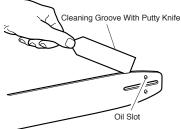
Figure 19 - Guide Bar Maintenance
